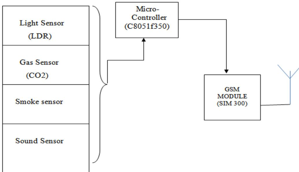
Figure 2: Block Diagram Transmission Side
